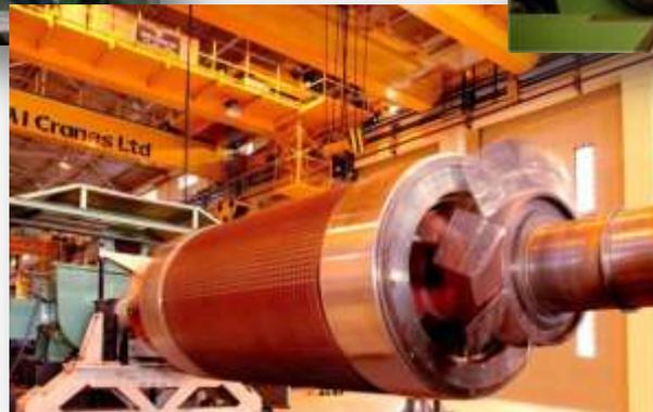
Dynamic balancing machine for rotor balancing
