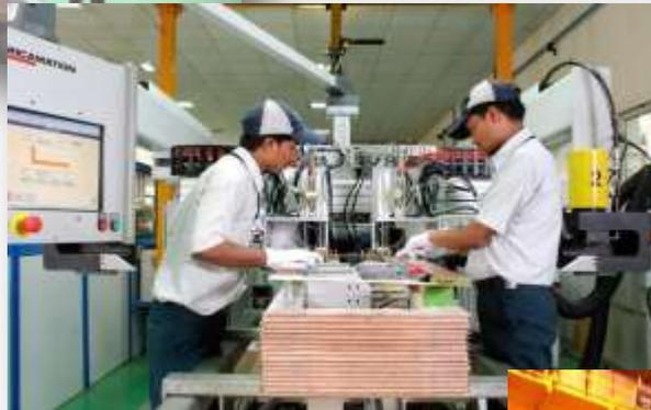
High precision brazing set up for rotor coils
