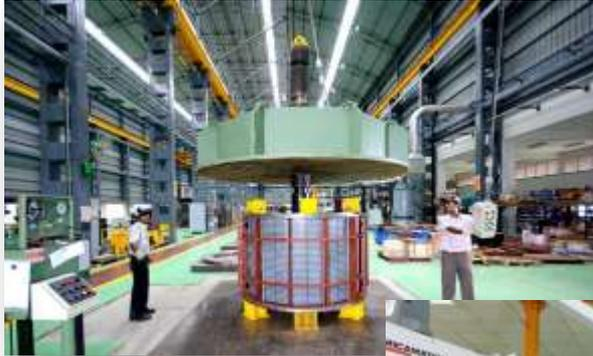
Horizontal vacuum pressure impregnation plant for stator
