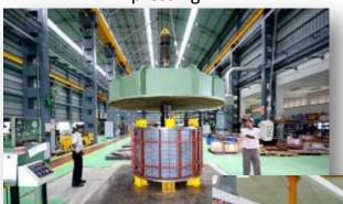
Horizontal vacuum pressure impregnation plant for stator
